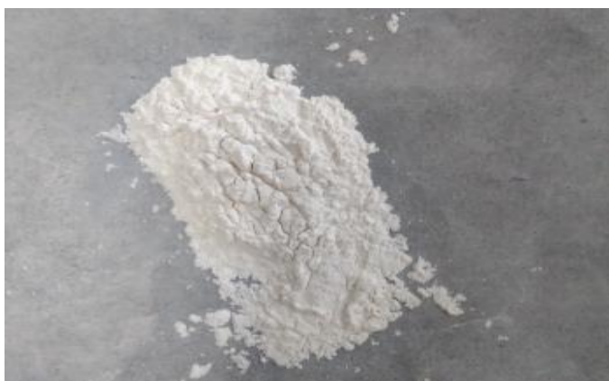
Figure 8: P molecular sieve prepared by coal fly ash.
