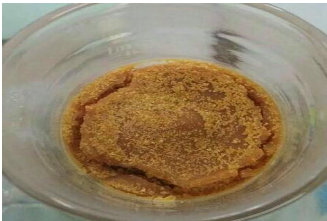
Figure 7: Residue of insoluble clinker after filtration.
