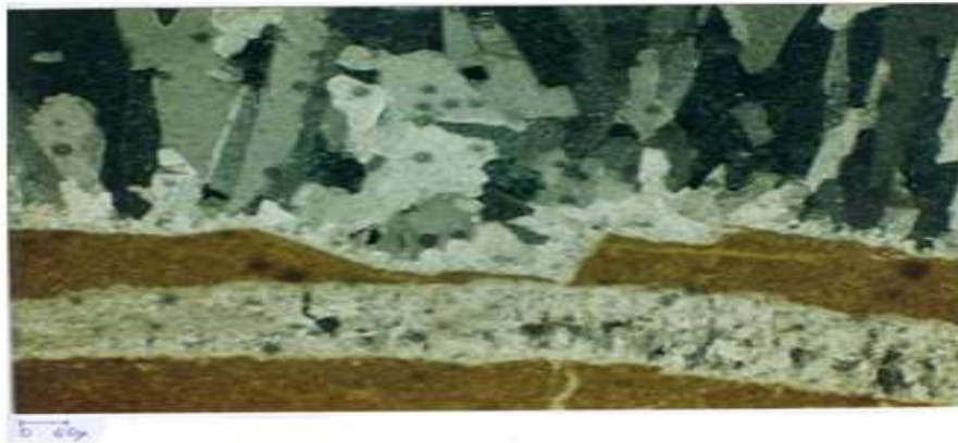
Figure 13: Crystals of increase isodiametric calcites from jagged edges in micritic limestone.
